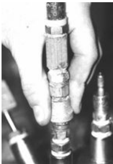
Figure 3.4 Disconnection of push on quick connectors
